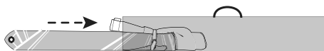
Fig. 10: Insert with the sleeve-end first into the sail bag and store horizontal.
