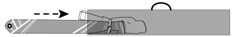
Fig. 9: Insert with the sleeve-end first into the sail bag and store horizontal.
